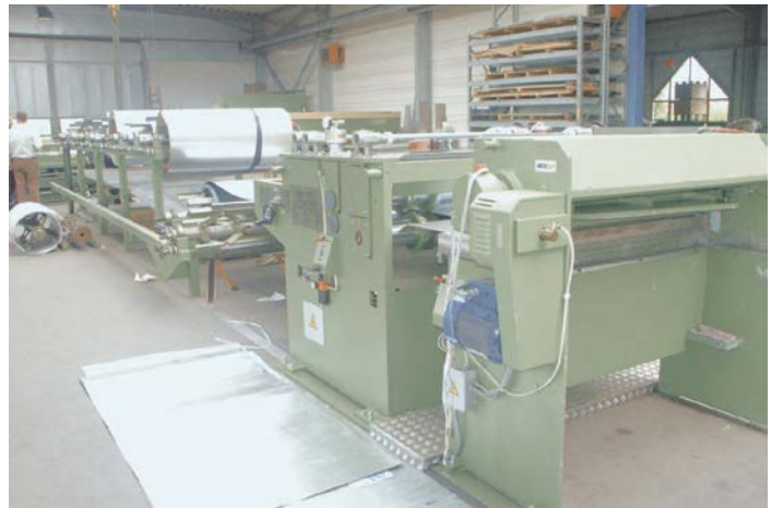
▲ The concept of roll-tooling and continuous feed are also utilized by other material-handling equipment, including levelers (that stretch and flatten material), cut-to-length lines, slitters and curving machines. Photos courtesy of Rob Haddock.
